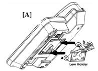
[A]: For the Holder fixed, you can follow the picture to do it. First, you need to fixed the Low Holder, the steps is from "a" to "b".
